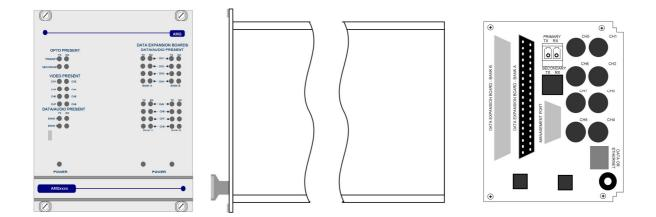
The **AMG4707AG-DR-SF** is a rackmount data transmit unit designed to transmit and receive up to 8 data or audio signals with Dual Redundant operation over two singlemode fibres. The 8 data/audio channel interfaces, whether RS232, RS422, RS485, 20mA, TTL, Contact Closure, Lonworks or Audio, are defined at manufacture by the addition of daughter boards fitted onto the Data Expansion Board A.
